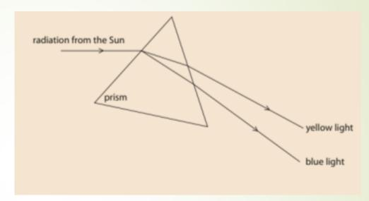
**Q25** State the phenomena observed in the above diagram. Explain with reference to the diagram, which of the two lights mentioned above will have the higher wavelength?
