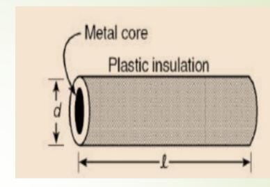
Q15 Plastic insulation surrounds a wire having diameter d and length l as shown above. A decrease in the resistance of the wire would be produced by an increase in the
