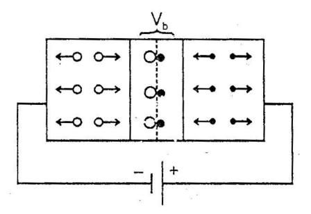
In reverse bias, holes and free electrons move towards negative and positive terminal of battery. So the width of depletion layer increases with increase in applied voltage upto certain limit.
