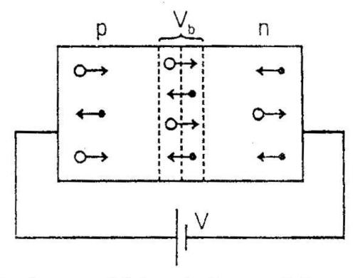
In forward bias, holes and free electrons start penetrating the junction, so width decreases with increase in applied potential.
