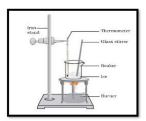
The setup shows melting of ice. For the first time interval  $t_1$ , the temperature gradually dropped. In the next time interval  $t_2$ , the temperature remained constant until all the ice melted. In the next time interval  $t_3$ , the temperature gradually increases.
